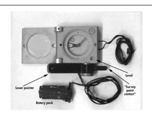
Figure 2 - 'Lasercompass' - geological compass with laser mounted on swivel attached - described in CP22
